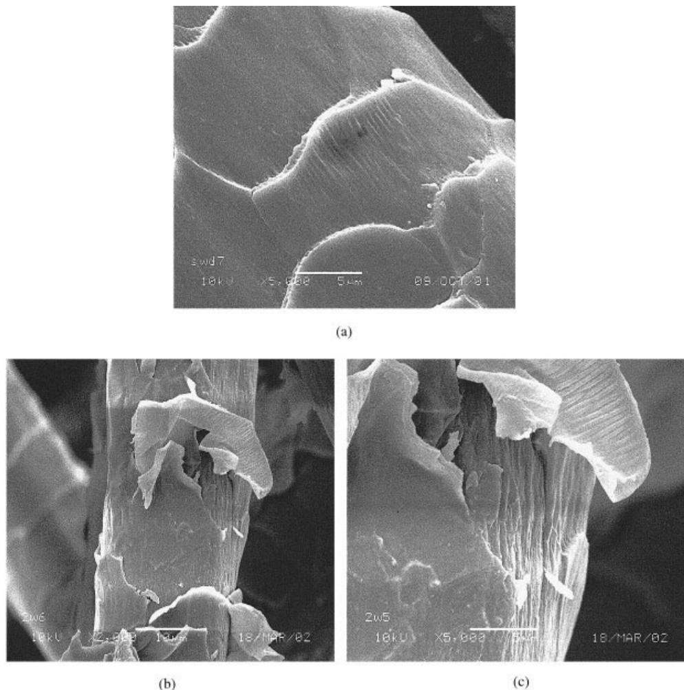
**Figure 4** Exemplary scanning electron micrographs of wool fibers: (a) untreated wool fiber and (b,c) wool fibers descaled in formic acid at 35°C for 1 h.
